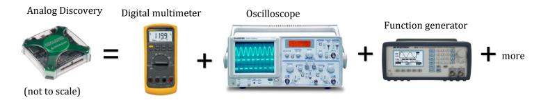
The Analog Discovery (AD) device we are using this semester has the functionality of several electronic devices (seen above). It is controlled by software.
