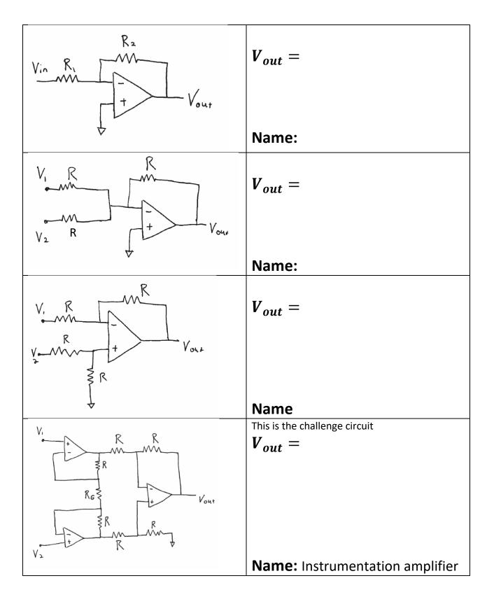
Now we ask you to **evaluate** two different op-amp configurations as shown in the figure below through measurements. You'll need a LMC6484 chip and an Analog Discovery. Build both circuits.
