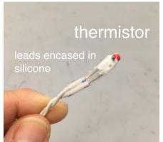
\*For the curious, thermistors are made of semiconductors. Thermal energy increases the number of electrons that are free to conduct; in semiconductors, as  $T\uparrow$ ,  $R\downarrow$ .
